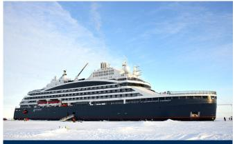
Le Commandant Charcot is currently the non-nuclear vessel with the most icebreaking capability in the world with its Polar Class 2 rating.
