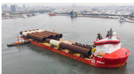
The transport vessels Audax and Pugnax, which were used to transport construction parts for LNG production facilities in the Arctic, are also an Aker Arctic design. Lately, the vessels have been used to transport towers and foundations to offshore wind parks. Photo: Yunlin Com_Taiwan
