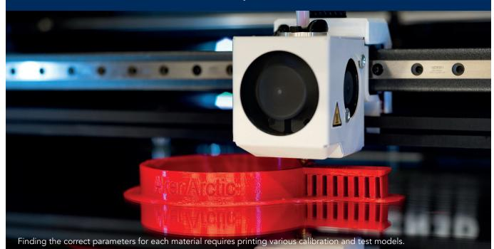
About a year ago, Aker Arctic acquired a 3D printer to investigate if certain parts for model testing and prototyping could be produced in-house to improve flexibility. The results have exceeded expectations.
