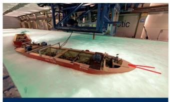
Close-coupled towing is a common way to escort commercial vessels in the Baltic Sea during winter. For the first time, close-coupled towing tests were performed in model-scale to compare different towing solutions.
