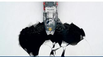
Full-scale tests with *Polaris* showed how a wide channel can be achieved with a narrower ship hull. The new icebreakers will be able to create channels of variable widths up to 32 metres.
