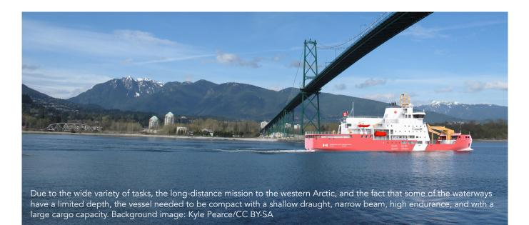
Aker Arctic's aspiration was to develop a concept design with a hull form which balanced icebreaking, seakeeping and open water performance, and was compact yet big enough to accommodate everything.
