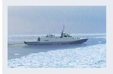
One of the recent propulsion packages ordered from Aker Arctic includes shaft lines and propellers for four new ice-going multi-role corvettes under the Finnish Defence Forces' Squadron 2020 project. A key challenge in the design was meeting the stringent low underwater noise requirements while maintaining high ice class performance.
