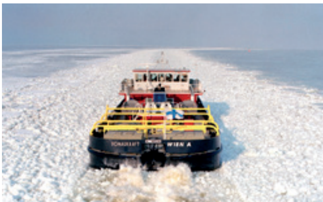
The river icebreaker Röthelstein opening a channel and managing brash ice on the Danube in Austria.
