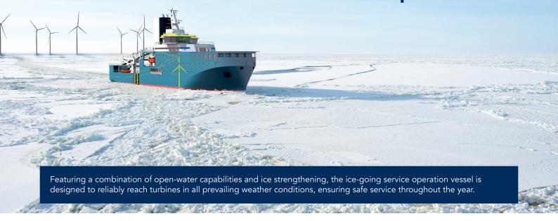
Aker Arctic's design team has finalised the concept for the first year-round service operation vessel (SOV) for seasonally freezing seas. The concept design can be tailored to a specific operational area and facilitates wind farms' investment calculations.
